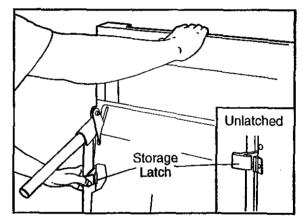
2. Hold the treadmill firmly with both hands, and lower the treadmill to the floor. Do not drop the treadmill frame to the floor. To decrease the possibility of injury, bend your legs and keep your back straight.
